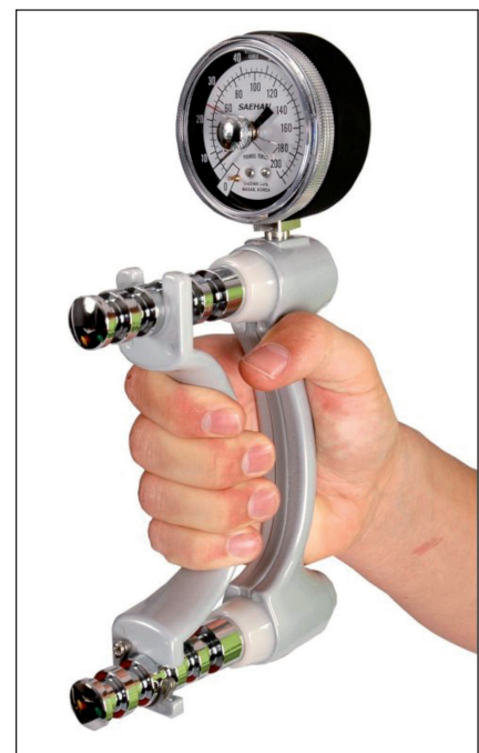
Figure 2. Dynamometer. Hand held instrument measures grip strength in kilograms and pounds. We used the average of five attempts per hand. Motivation and fatigue are factors requiring clinical support during testing to elicit maximum performance.
